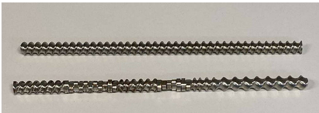
Figure 3.3 Screws used in hot melt extrusion. Top: Conveyor screw. Bottom: Screw with additional kneading and melting elements.
