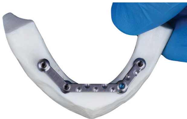
Fig 5 Modified Sheffield Test: All screws were removed except for the one in position 32.
