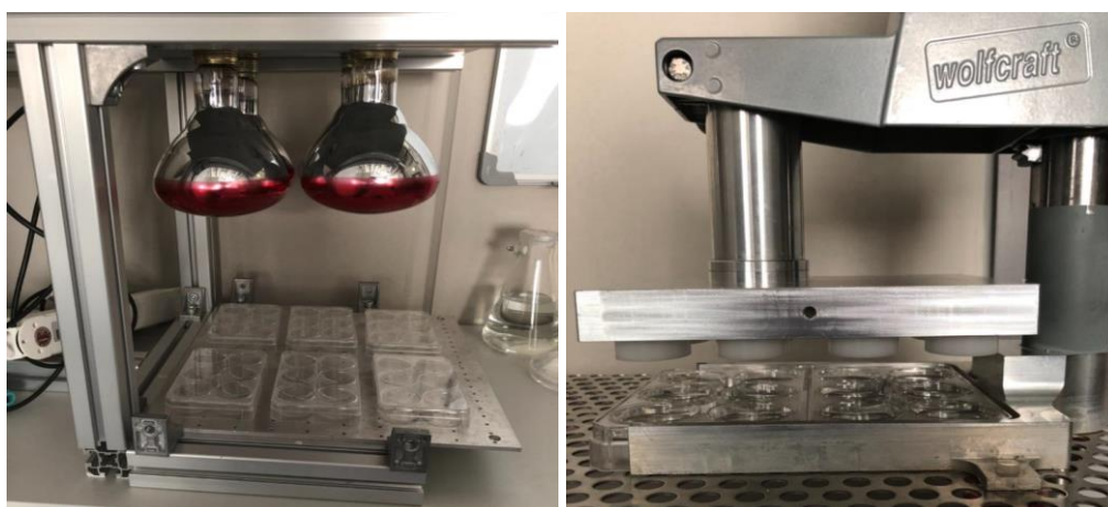
Figure 16: Membrane curing setup (R) with the custom metal stamping device with the transfer tool (L)
