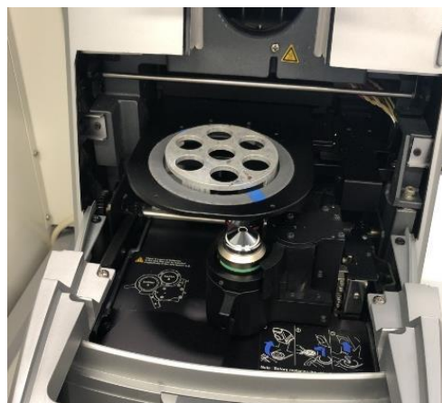
Figure 21: KEYENCE Fluorescence Microscope with the custom CellDrum™ holder
