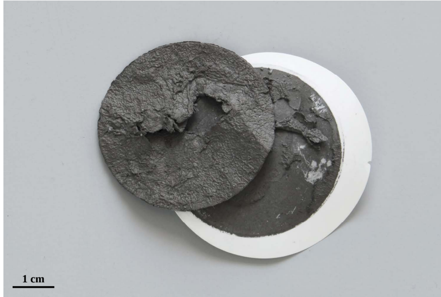
Figure 5.17: Digital photograph of the precipitated W nanowire “fleece” partially removed from the filter paper. Close-up views of these nanowires are shown in fig. 5.18.
