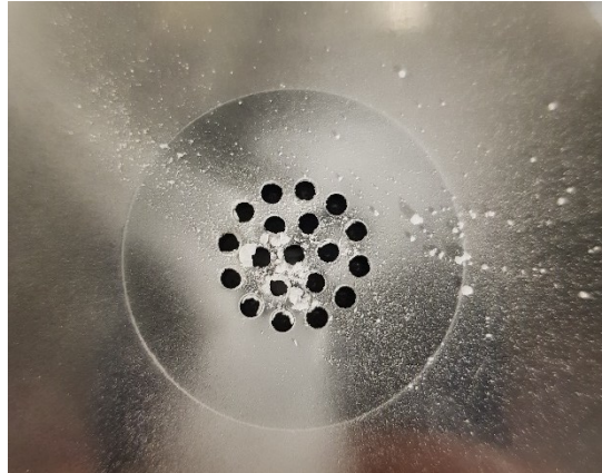
Figure 29: Picture of the multi-tip die after external lubrication on the Styl'One compaction simulator with a high spray rate
