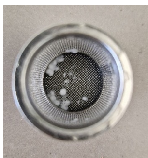
Figure 71: Picture of the residues in the dissolution basket after 60 min dissolution test (Ludiflash® ODMTs with 40% NPX and 5% SSF)
