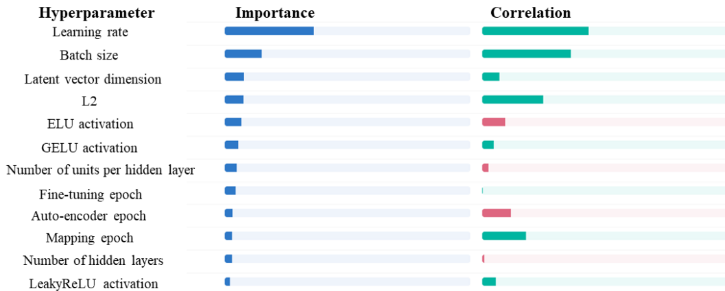
Figure 6.7: Hyperparameter importance and their correlations with validation loss. Left: importance quantifying each hyperparameter's contribution to the variability of the validation loss. Right: correlation with the validation loss.
