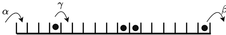
Fig. B.11. A schematic representation of the Totally Asymmetric Simple Exclusion Process (TASEP) on a single segment. Particles enter on the left with entrance rate \alpha from an infinite reservoir, step along the segment with excluded-volume interactions with a rate \gamma , and leave the segment on the right with exit rate \beta to an infinite reservoir.
