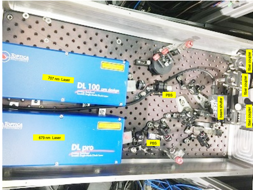
(a) Photo of the distribution breadboard of the repump lasers.
