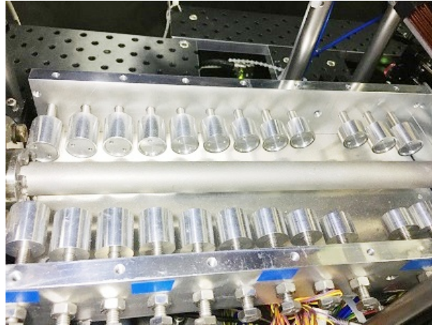
Figure 3.5: The photo of Zeeman slower which is based on a 2-D array of neodymium permanent magnets with transverse field.
