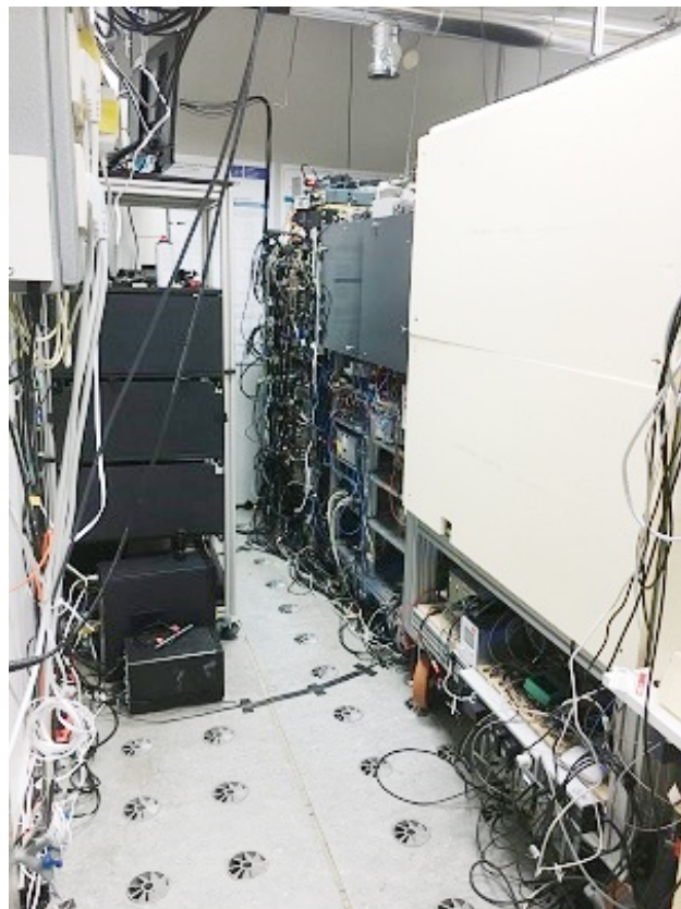
Figure 3.2: The SOC2 optical clock currently (2024), still at PTB, in the same laboratory space. In the foreground right is the enclosed new clock laser. The atomics package is at the center, covered with black panels. On the left is a rack containing laser subsystems.
