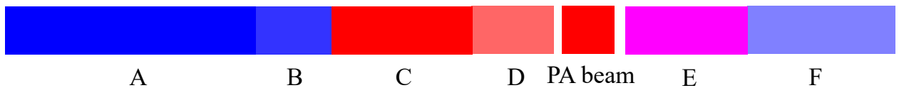
Figure 6.11: The timing sequence of clock operation with PA beam. From phase A to D, atoms are cooled down and loaded into the optical lattice. Then, a PA beam that is on resonance with the PA line which is \sim 222 MHz detuning from the ^1S_0 \leftrightarrow ^3P_1 transition is delivered into the lattice. E and F are the interrogation and detection phases. More details of A to F in Figure 3.21.
