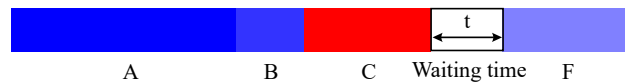
(c) The timing sequence of TOF measurement of broadband red MOT. A: atoms loading and blue MOT, B: low-power blue MOT, C: broadband red MOT, F: detection; more details in Figure 3.21.
