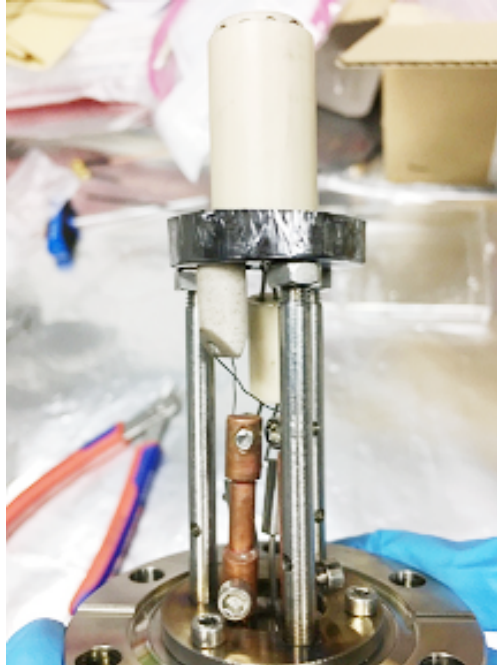
(a) The atomic oven installed on a CF35 flange.
