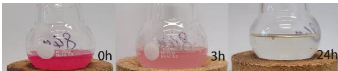
Figure 84: Colour progression of the IEDDA click reaction between compound P15 and dienophile 24 ,
