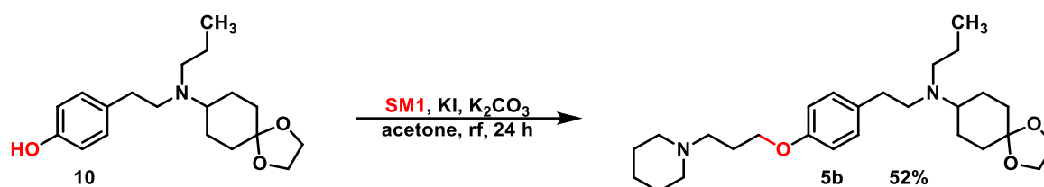
Figure 49: Reaction of the alkylation of compound 10 with SM1 under Finkelstein conditions, yielding compound 5b .
