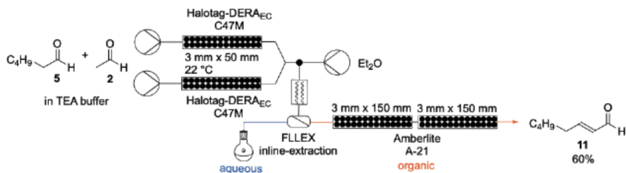
Figure 6: Experimental set-up of the continuous flow mode two-step synthesis of \alpha,\beta -unsaturated aldehyde ( E )-octenal (11).
