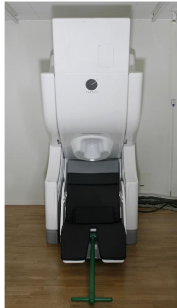
Figure 1. MEG setup. 306-channel MEG system (MEGIN) in a magnetically shielded room at the University hospital Düsseldorf. MEG sensors are cooled by liquid helium which is stored in the dewar.
