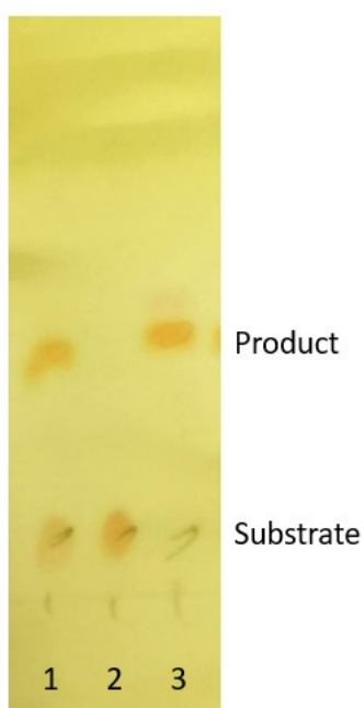
Figure S 58: TLC colored with Moly-Dip of the allylation reaction with SgMT. 1: Conditions by Diana Amariei (pre-incubation of AchMT, SAH ( 94 ) and allyl iodide before adding SgMT and the cWW 3a ), B: negative control (condition of Diana Amariei without HMT), C: direct recycling conditions.
