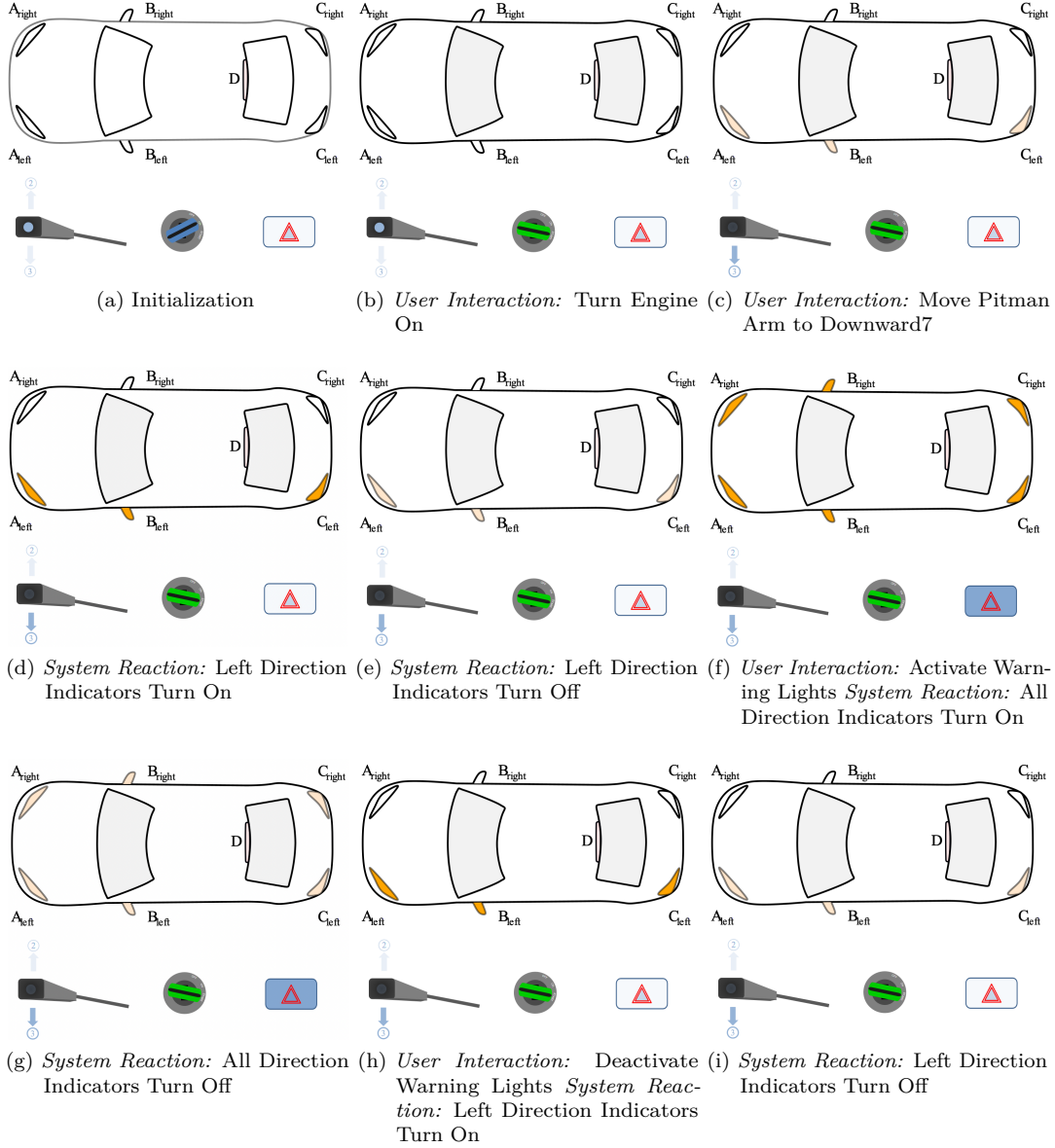
Figure 3.7.: Validation of ELS-1 , ELS-8 , ELS-12 from User's Perspective in ProB2-UI (Visualization and User Interaction in VisB, System Reaction via SimB)
