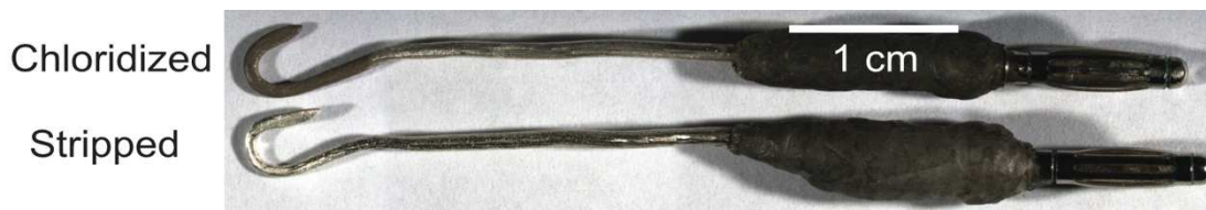
Figure 3. Surface silver chloride electrode. Top: freshly chloridized (see the dark hook), bottom: freshly stripped electrode (see lustrous hook).
