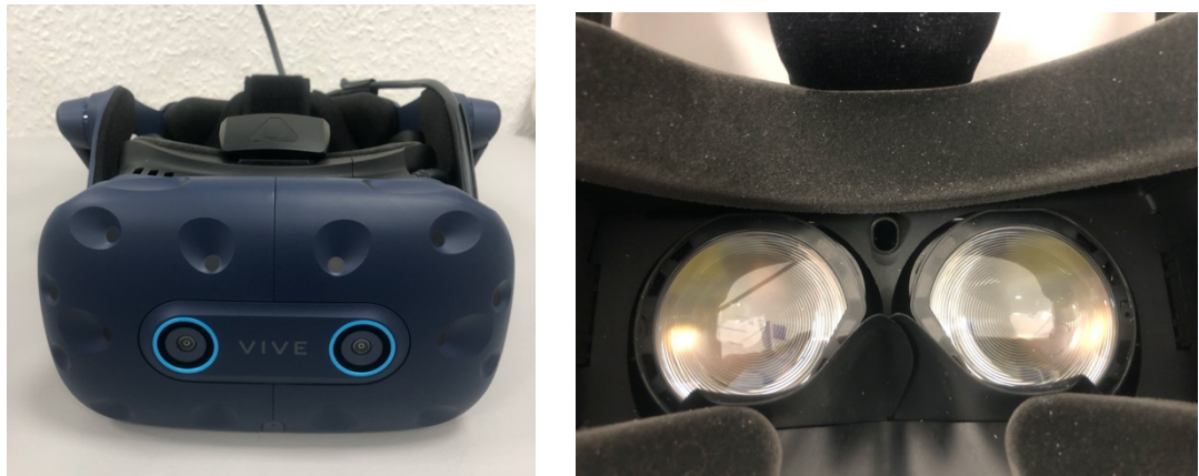
Figure 7. HTC Vive Pro Eye headset with built-in Tobii eye tracker. The eye-tracking cameras and infrared illuminators are positioned around the lenses inside the headset, allowing them to monitor eye movements. Photo by author.
