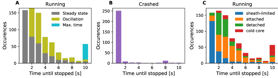
Figure 7.5: Histograms of the total runtime of non diverging (A, C) and diverging/crashing (B) simulations. A: The colors denote the different conditions that stopped a simulation. Such are reaching a steady state (grey), showing stable oscillations (olive) or reaching the maximum runtime (cyan). C: The colors denote the different physical regimes seen in the simulations. The classifications into the four regimes sheath-limited (blue), attached (orange), detached (green) and cold core (red) is performed based on the criterion introduced in Section 7.4. This analysis is conducted on half of the simulations in the test set, as only for these simulations the exact timings were recorded.
