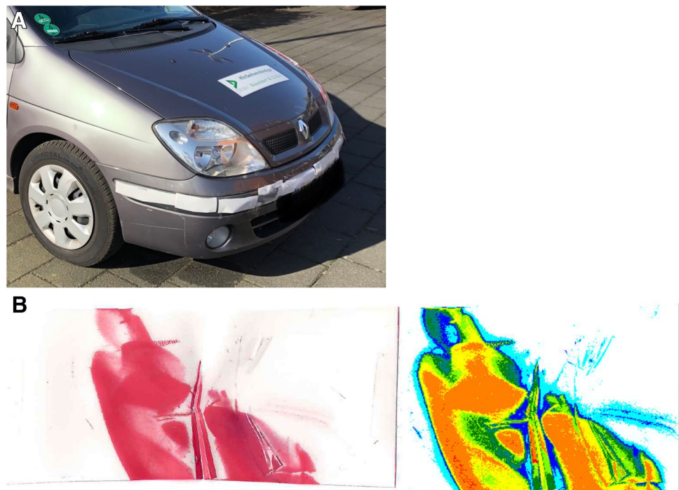
Fig. 2 a Example of the film being applied to the front bumper of one of the test cars. b Fujifilm prescale (MS) pressure film after impact (left) and after digital evaluation (right)
