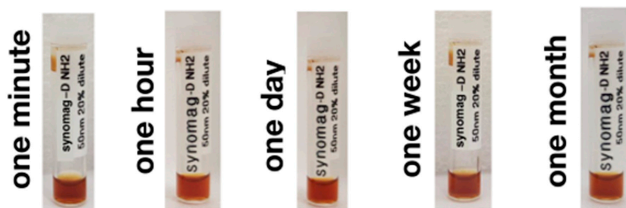
Figure S2. Qualitative assessment of the colloidal stability for synomag nanoparticles over time from 1 min up to 1 month.
