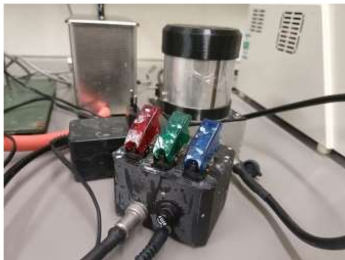
Figure 15. The self-built photoreactor used for the photocatalytic perfluoroalkenylations
