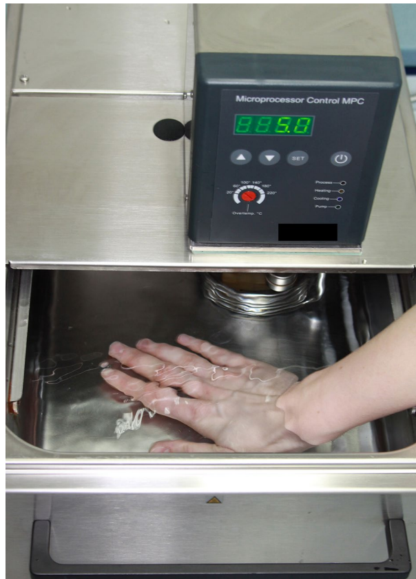
Figure 2. Circulating water bath system for the cold pressor test with immersed right hand. The water temperature was a constant 5 °C throughout the basin.
