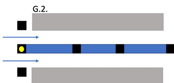
Fig. 2 G.2; alley drive with an upstream light signal indicating which of the two lanes should be used
