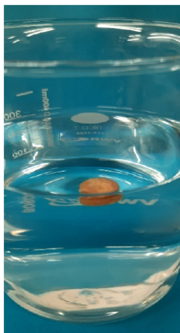
Figure 7. Floating properties of PP1 in 300 mL 0.1 N HCl, 37 \pm 0.5 \text{ }^\circ\text{C} .
