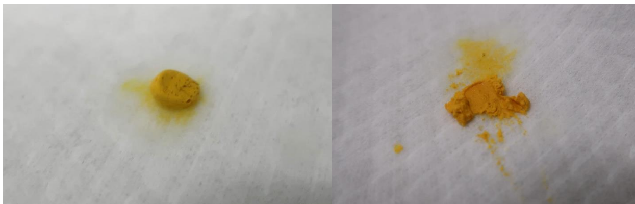
Figure 13: Peposertib tablet after dissolution. Left: After taking the tablet out of the vessel. Right: After crushing with a spatula
