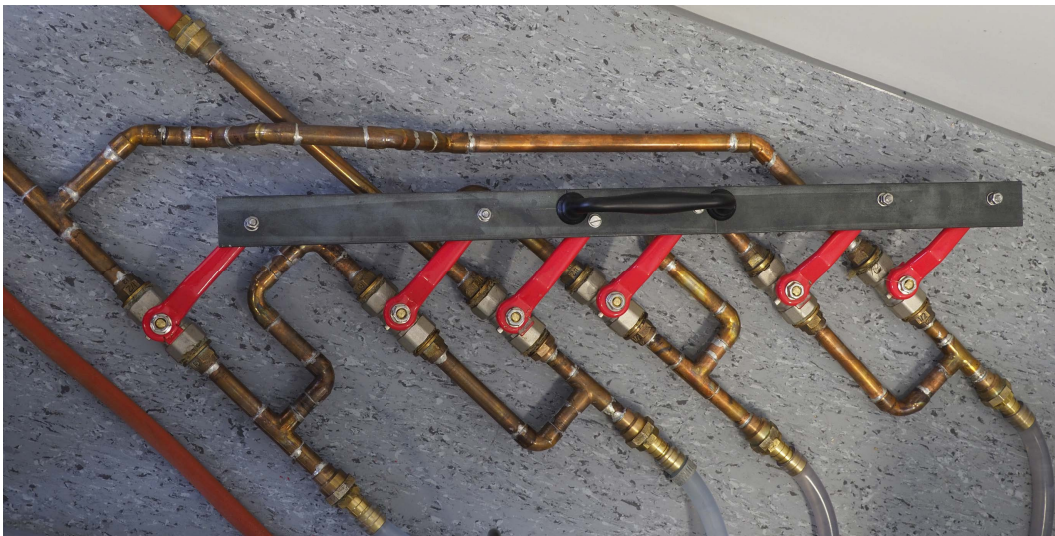
(b) Photographic image of the switching valve. Please note that the ball valves used in the assembly have been modified, so the handle does not indicate the switching direction correctly.
