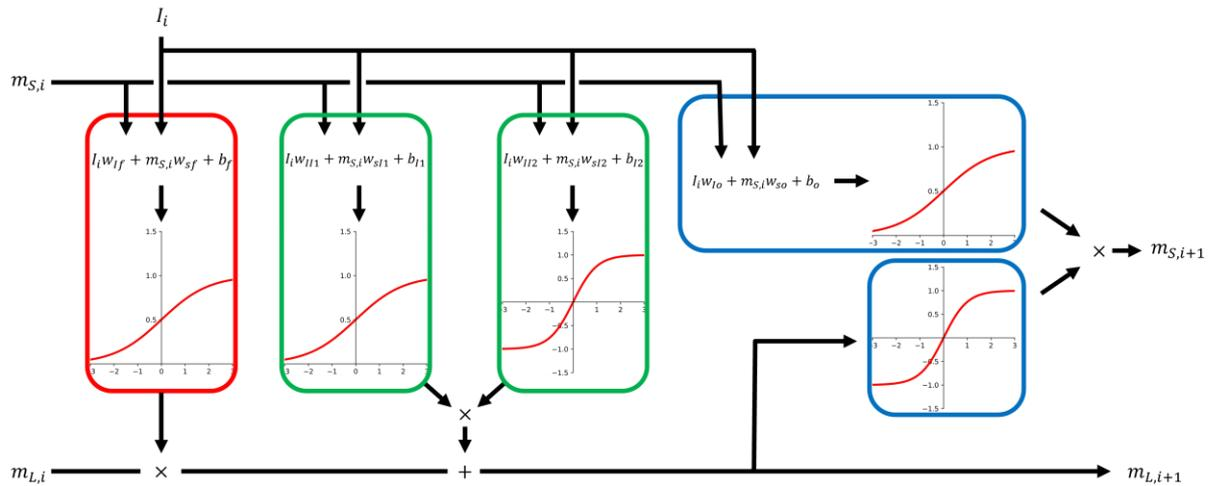
Figure 12: Long short-term memory (LSTM) layer, red box: forget gate, green boxes: input gate, blue boxes: output gate, multiplication operations for results of activation functions are given as  $\times$ , additions as  $+$
