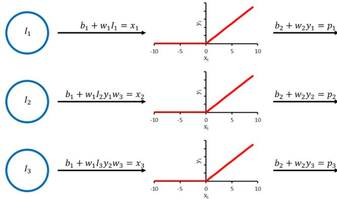
Figure 11: Unrolled recurrent layer with a data series of length 3 as the input and ReLU activation function
