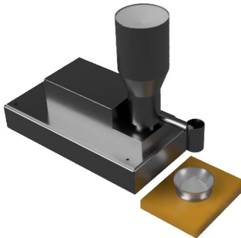
*Figure 2: Flat-bottom dosing unit and external catch scale; sketch made using Autodesk Fusion 360*
