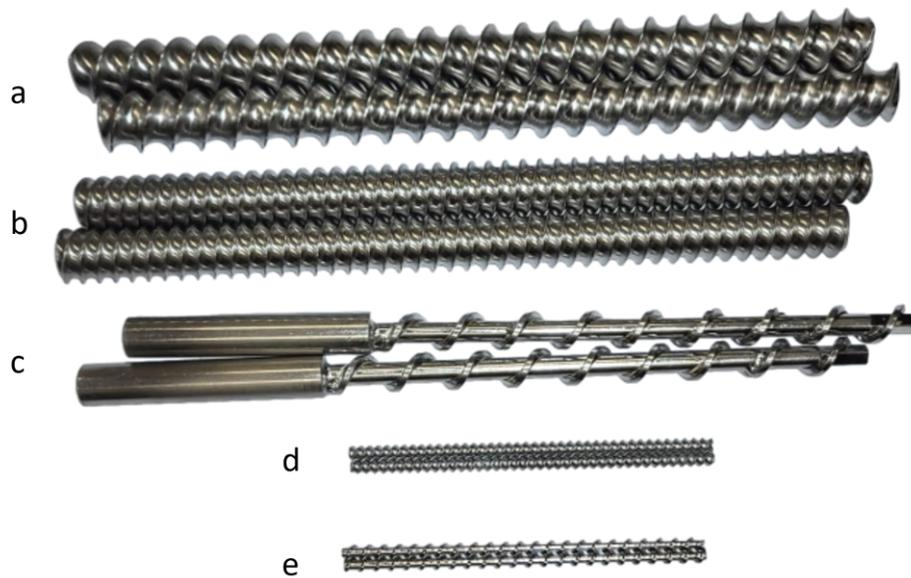
Figure 1 a-c: Dosing screws of a diameter of 20 mm, a: wide pitch double-flight intermeshing, b: narrow pitch double-flight intermeshing, c: single-flight non-intermeshing, d and e: dosing screws of a diameter of 5 mm, d: double-flight intermeshing, e: single-flight intermeshing with conical shafts
