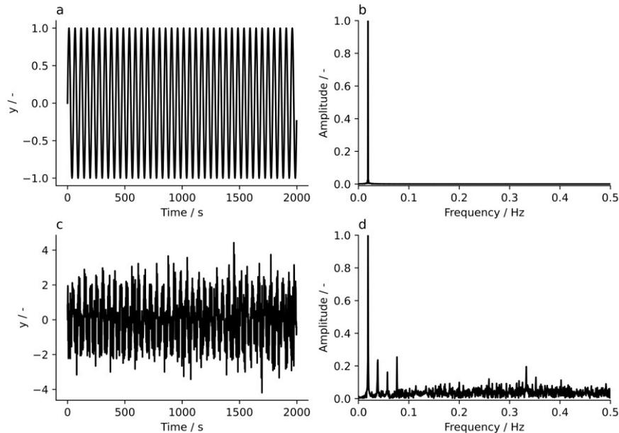
Figure 6: Time (a and c) and frequency (b and d) domain of an ideal sinusoidal and measured data of the frequency of 0.019 Hz.
