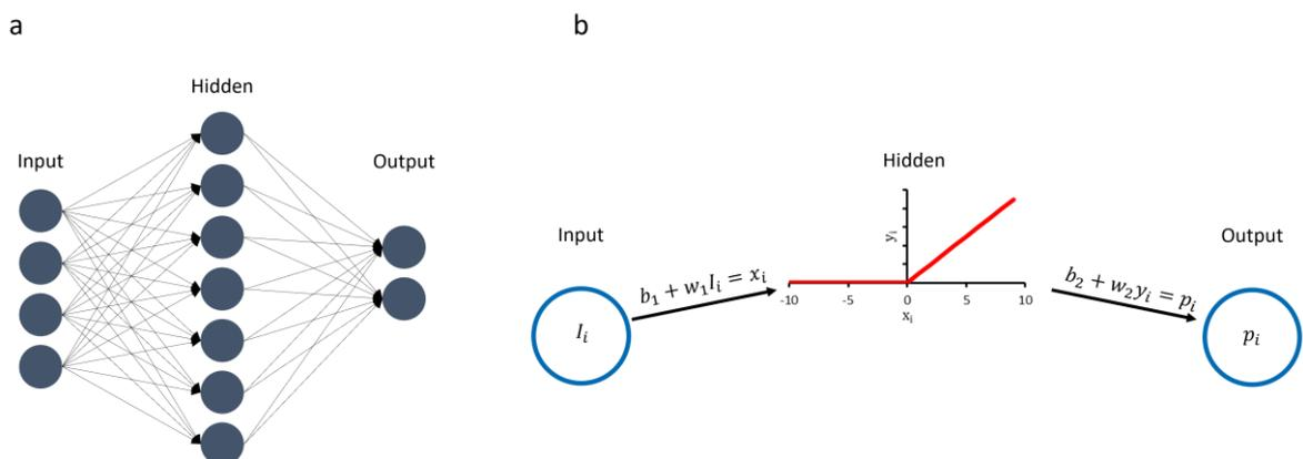
Figure 8 a: The structure of a simple neural network, b: depiction of a basic mathematical function model for the nodes and the connections.
