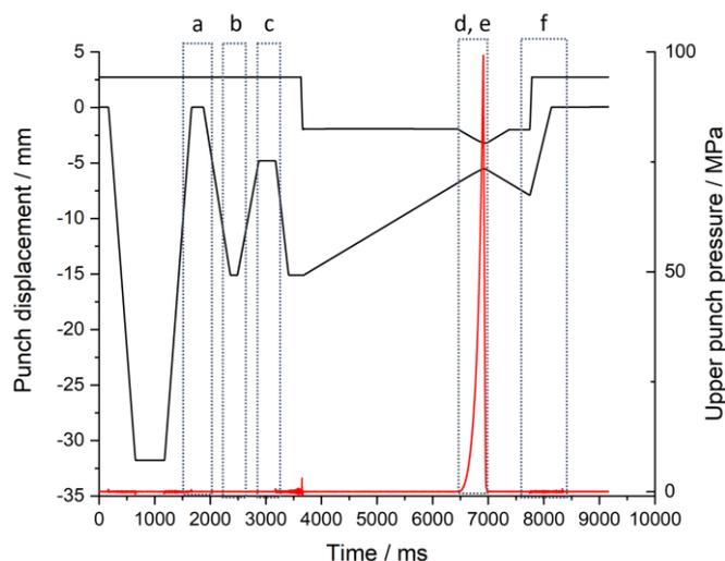
Figure 3: Example of data of a tableting process, black: punch displacement, red: compression pressure measured at the upper punch, a: external lubrication, b: die filling, c: dosing, d: compression, e: decompression, f: ejection of the tablet
