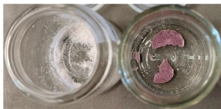
Figure S35. Powder of 5 before (left) and after (right) pressure (9 t, 10 min).
