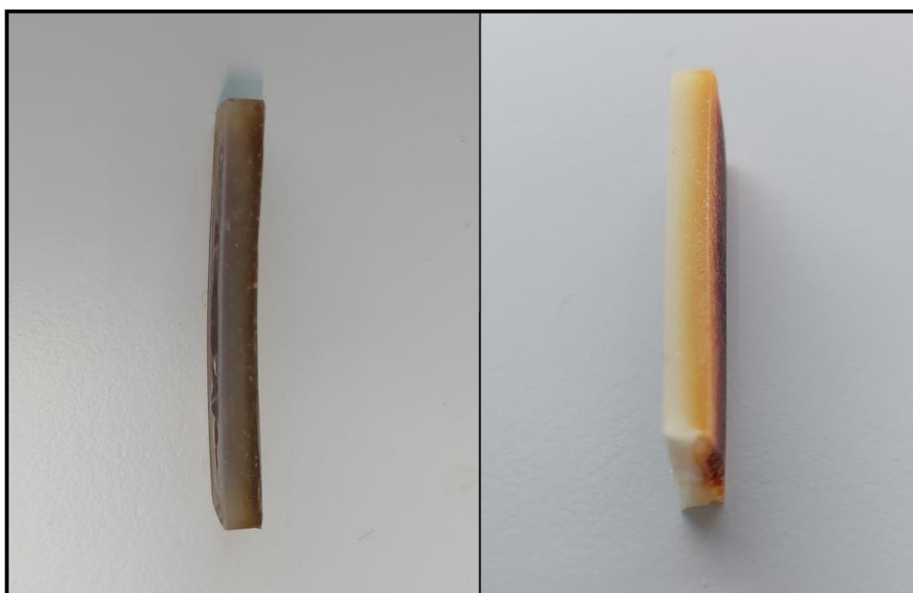
Figure 3.23: Cured samples of formulation F-HAE. Left: Shortly after curing. Right: After one week of storage. A distinct discoloration takes place: the material becomes brighter over time. In the right picture, an attenuated discoloration gradient can be seen on the inside of the sample.
