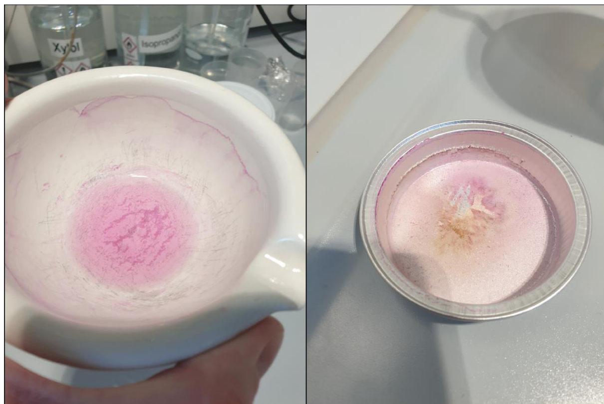
Figure 3.38: p(4-vinylphenol) and sodium hydrogen sulfate monohydrate were grinded with pestle and mortar. Left: Dispersion in acetone. Right: After solvent evaporation.
