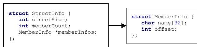
Fig. 3. Metadata structs used to map proxy object fields onto native C struct fields.
