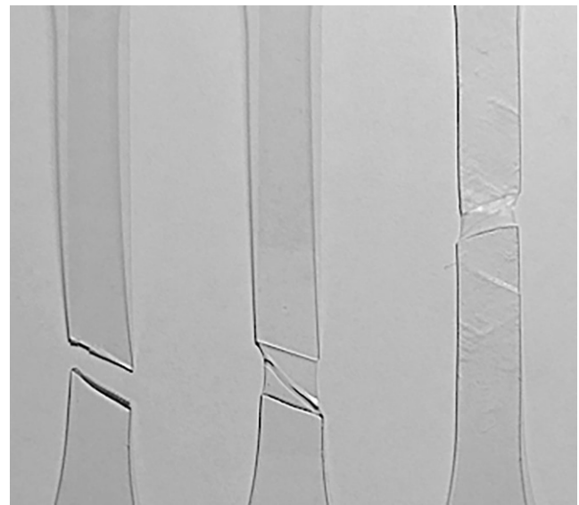
Fig. 9 Specimen after tensile testing (left to right: sudden fracture, i.e., brittle fracture behavior; necking, i.e., ductile fracture behavior; finger-printed specimen with streaking and multiple locations of necking)
