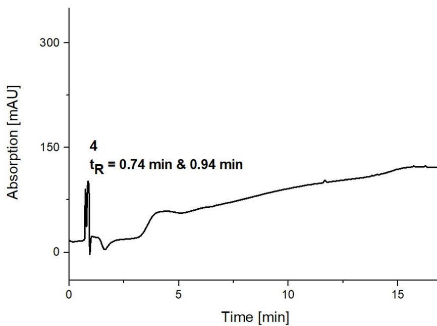
**Figure S17:** RP-HPLC chromatogram of **4**, linear gradient from 5 to 95 vol% acetonitrile in water (+ 0.1 vol%  $\text{HCOOH}$ ) in 15 min then 2 min isocratic at 95 vol% acetonitrile in water.
