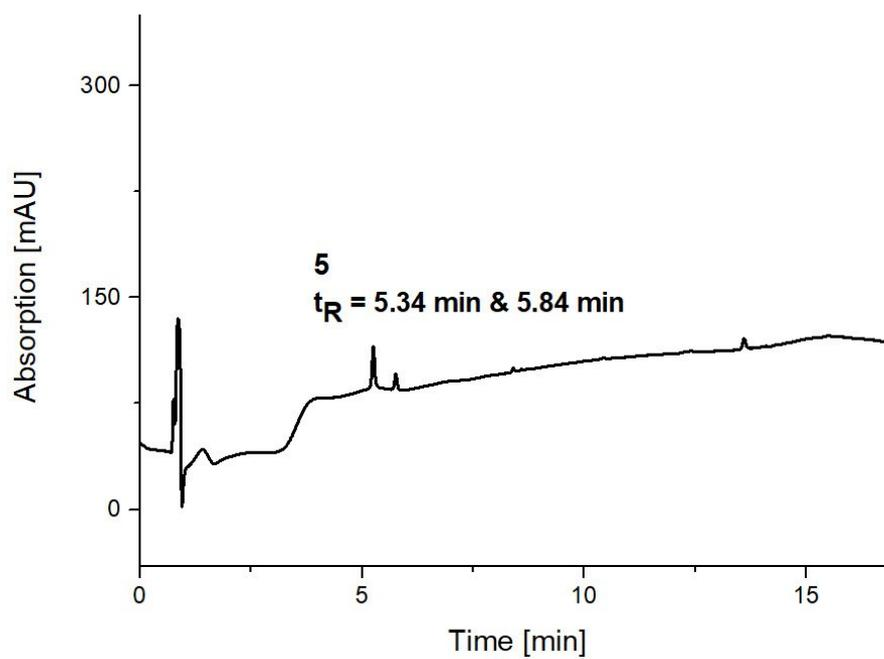
**Figure S21:** RP-HPLC chromatogram of **5**, linear gradient from 5 to 95 vol% acetonitrile in water (+ 0.1 vol% HCOOH) in 15 min then 2 min isocratic at 95 vol% acetonitrile in water.
