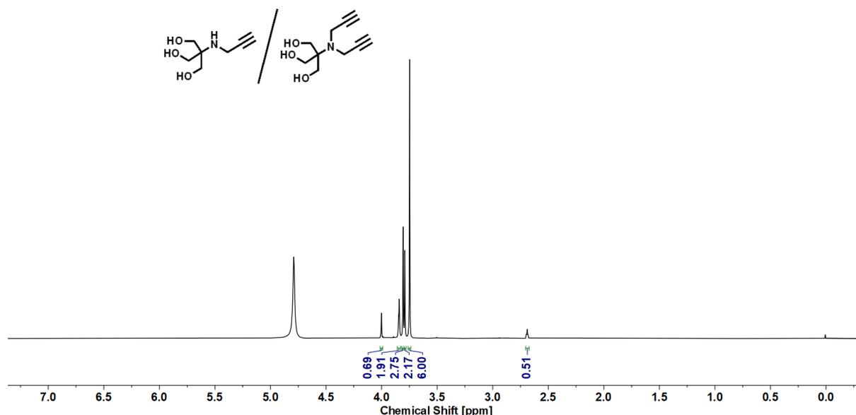
**Figure S15:** <sup>1</sup>H NMR spectrum of **4** (300 MHz, D<sub>2</sub>O).
