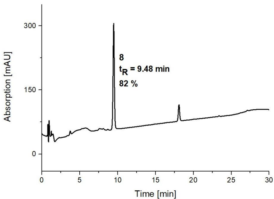
**Figure S37:** RP-HPLC chromatogram of **8**, linear gradient from 5 to 50 vol% acetonitrile in water (+ 0.1 vol% HCOOH) in 30 min.
