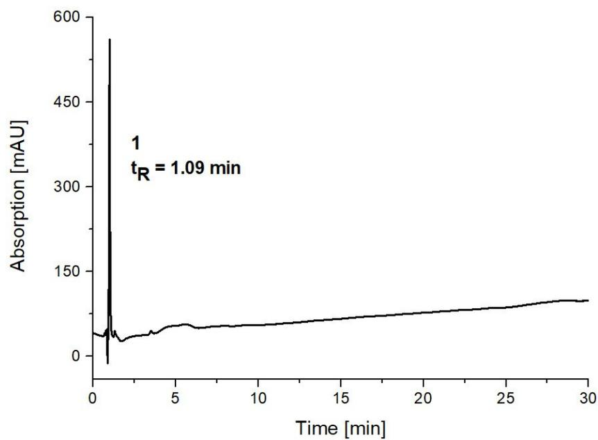
**Figure S4:** RP-HPLC chromatogram of 1, linear gradient from 5 to 50 vol% acetonitrile in water (+ 0.1 vol%  $\text{HCOOH}$ ) in 30 min.
