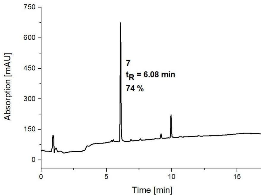
**Figure S32:** RP-HPLC chromatogram of **7**, linear gradient from 5 to 95 vol% acetonitrile in water (+ 0.1 vol% HCOOH) in 15 min then 2 min isocratic at 95 vol% acetonitrile in water.
