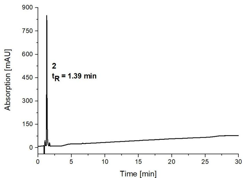
**Figure S9:** RP-HPLC chromatogram of **2**, linear gradient from 5 to 50 vol% acetonitrile in water (+ 0.1 vol% HCOOH) in 30 min.
