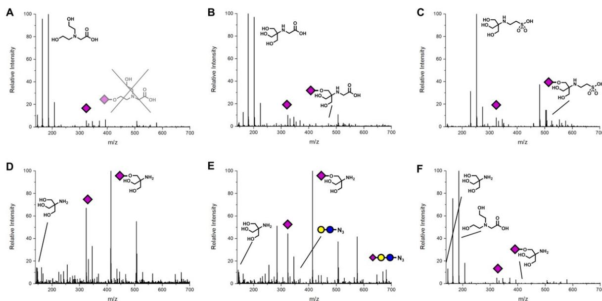
**Figure 19:** Mass spectra of enzymatic sialylation reactions using PmST1 P34H/M144L, **A:** 200 mM bicine (negative control), **B:** 200 mM tricine, **C:** 200 mM TES, **D:** 200 mM Tris, **E:** 11 mM LacN<sub>3</sub> in 200 mM Tris buffer (positive control), **F:** 11 mM Tris in 200 mM bicine buffer.
