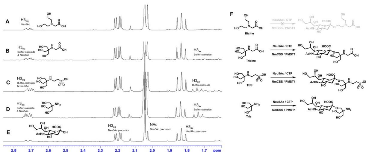
**Figure 18:** <sup>1</sup>H NMR spectra of enzymatic sialylation with Good's buffers using NmCSS/PmST1 WT (A-D), **A:** 100 mM bicine (negative control), **B:** 100 mM tricine, **C:** 100 mM TES, **D:** 100 mM Tris (positive control), **E:** 16.5 mM Neu5Ac (reference), **F:** enzymatic buffer sialylation using NmCSS/PmST1 method.<sup>[592]</sup>
