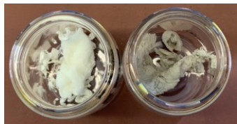
Figure 54: Aero gel before (left) and after (right) being exposed to ultrasound. Due to decomposition the brown colour can be observed.
