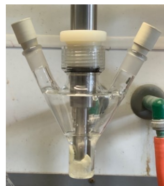
Figure 55: Sonochemical apparatus. The hydrogel was submitted into the suslick vessel and dissolved during the sonication process.
