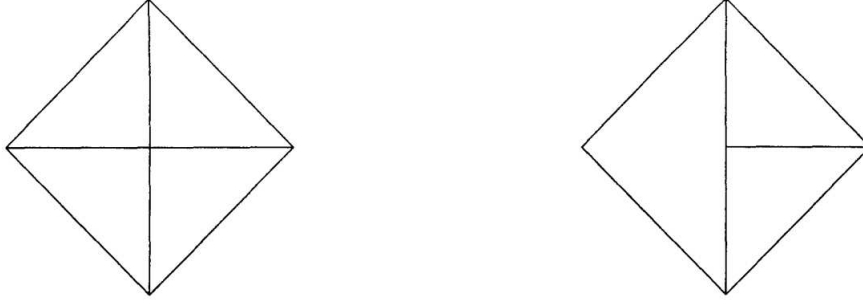
Figure 3.4: Two subdivisions: the one on the left is a valid triangulation and the one on the right is not because of the hanging node in the center. Figure from Ref. [10].
