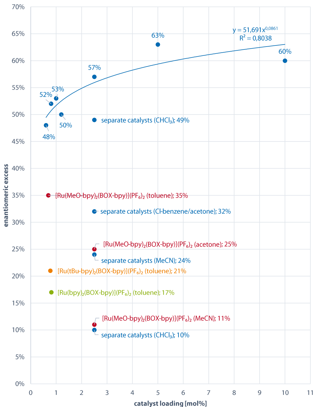
figure 43. Graphical representation of the dependency of the enantiomeric excess on asymmetric catalyst loading, along with other screening results of both the separate catalyst system (blue) and the bimetallic asymmetric photoredox catalysts 532 (green), 536 (yellow) and 537 (red) in different solvents.
