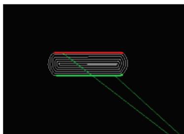
Figure 1. Detail from the watermark-embedding process. The side length (green + red) is recognized without the roundings and is encoded with bits.
