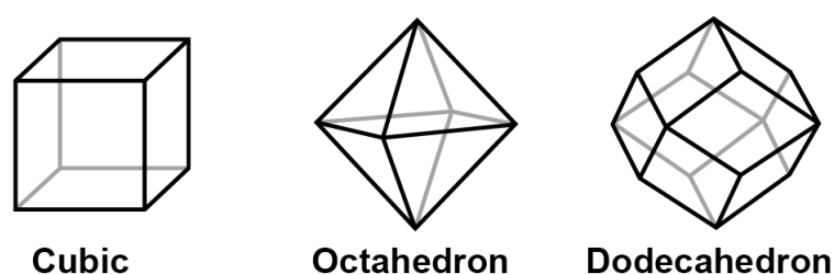
Figure 2.5.: Typical box types used in MD simulations of biomolecular systems.
