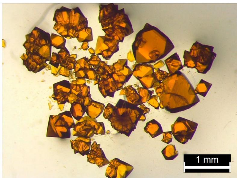
Figure S8. Crystals of  $[\text{Zn}(\text{lsa-az-tmpz})] \cdot \sim 1-1.5 \text{ DMF}$  obtained from a single crystal synthesis.
