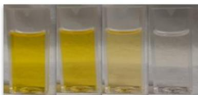
**Figure 14:** Depiction of the degradation of  $\beta$ -carotene within the model reaction using a surfactant-like alizarin derivative.
