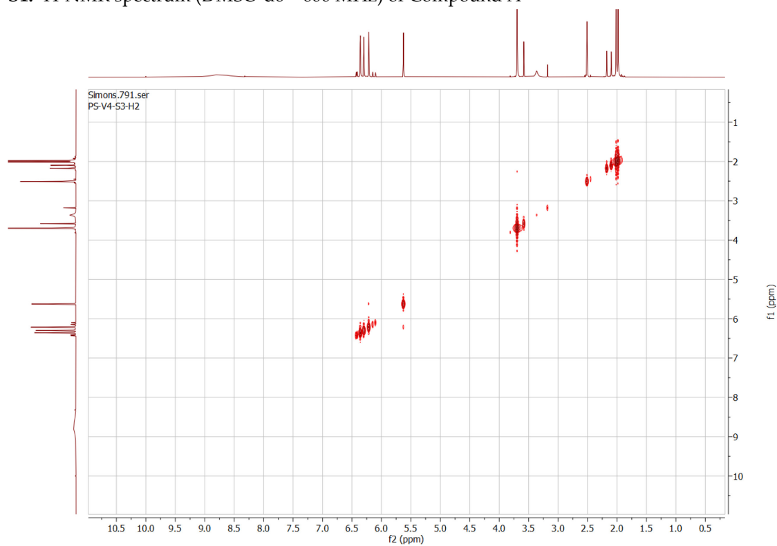
S2. COSY NMR spectrum (DMSO- \text{d}_6 – 600 MHz) of compound A
