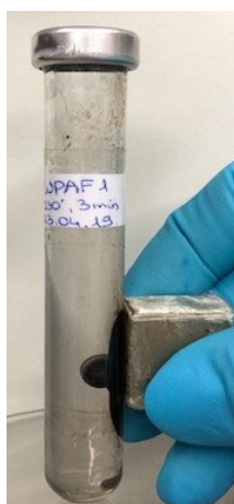
Fig. S51 Photos demonstrating the ferromagnetism of the Pd/Fe 3 O 4 -on-ZIF8-NP after washing in the MW-tube via the action of the magnet (the black layer near the cube-shaped magnet is the sample with the magnetic stirring bar on top of it). The photo is taken on a sample under inert atmosphere, but the ferromagnetism is retained in the air for days at least (seemingly indefinite time).
