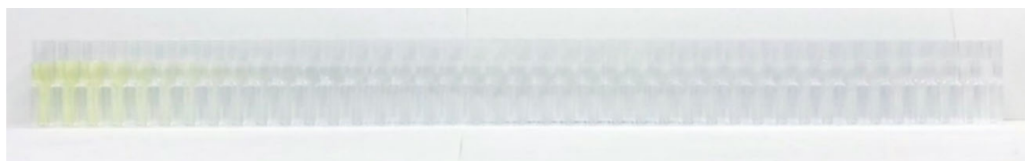
Fig. S88 An example sequence ( n \times 1 min) of spectrophotometric cuvettes with the diluted reaction medium. The yellow coloration, gradually disappearing in the course of the reaction, is conditioned by 4-nitrophenol.
