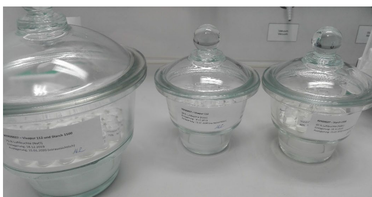
Figure 5-11: Desiccators containing the powder samples and the saturated salt solutions.
