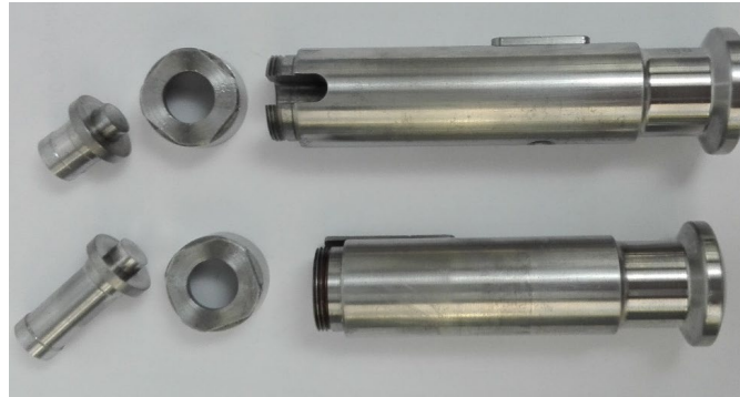
Figure 5-3: Punch set used for transverse KIM measurements including removable punch tips.
