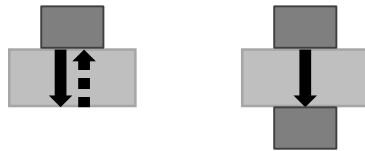
Figure 1-2: Schematic depiction of the pulse-echo (left) and pitch-catch (right) measurement set-ups. Solid arrow: transmitted signal, dashed arrow: reflected echo signal.
