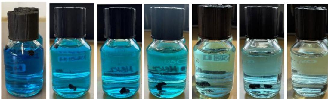
**Fig. S15** MB adsorption kinetics of MIL-53(Al)@Pine-MA (50 ml MB solution with 5 mg L<sup>-1</sup>). From left to right: start, 1 h, 2 h, 8 h, 24 h, 32 h, 48 h.
