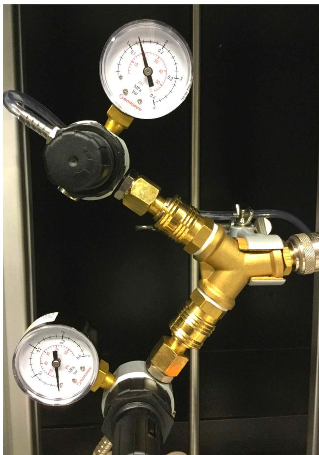
Figure 3.13: Adjustable pressure valves attached to inlet phase syringes on the other end.
