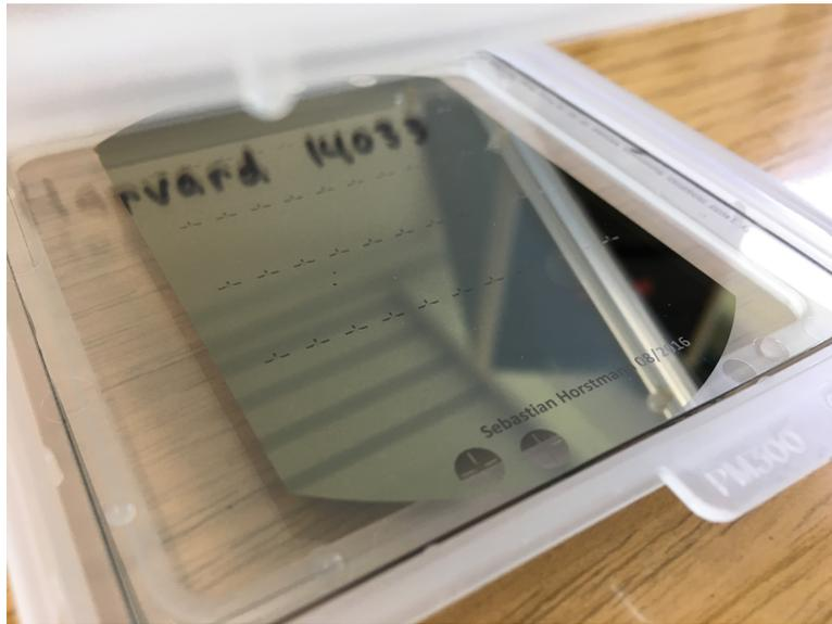
Figure 3.16: High-precision chrome photomask holding only the cross flow junction features critical for femtoliter droplet formation.
