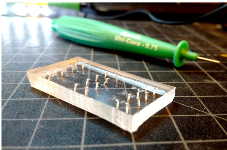
Figure 3.9: Microfluidic chip's PDMS stamp after step (l) and before bonding to glass.
