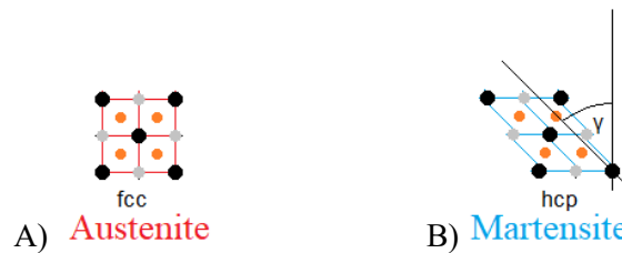
Fig. 8: Changes in the crystal structure of a superelastic alloy.
