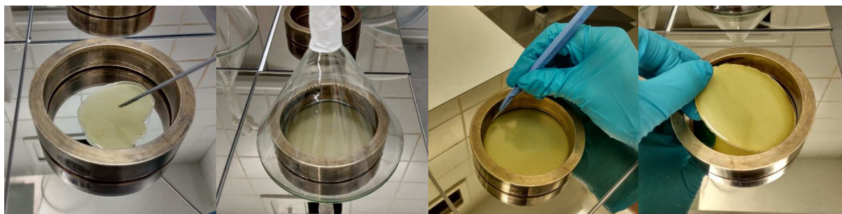
Figure S24. Preparation of membranes by solution casting (from left to right): casting the solution, drying, cutting with a scalpel and removing the membrane.
