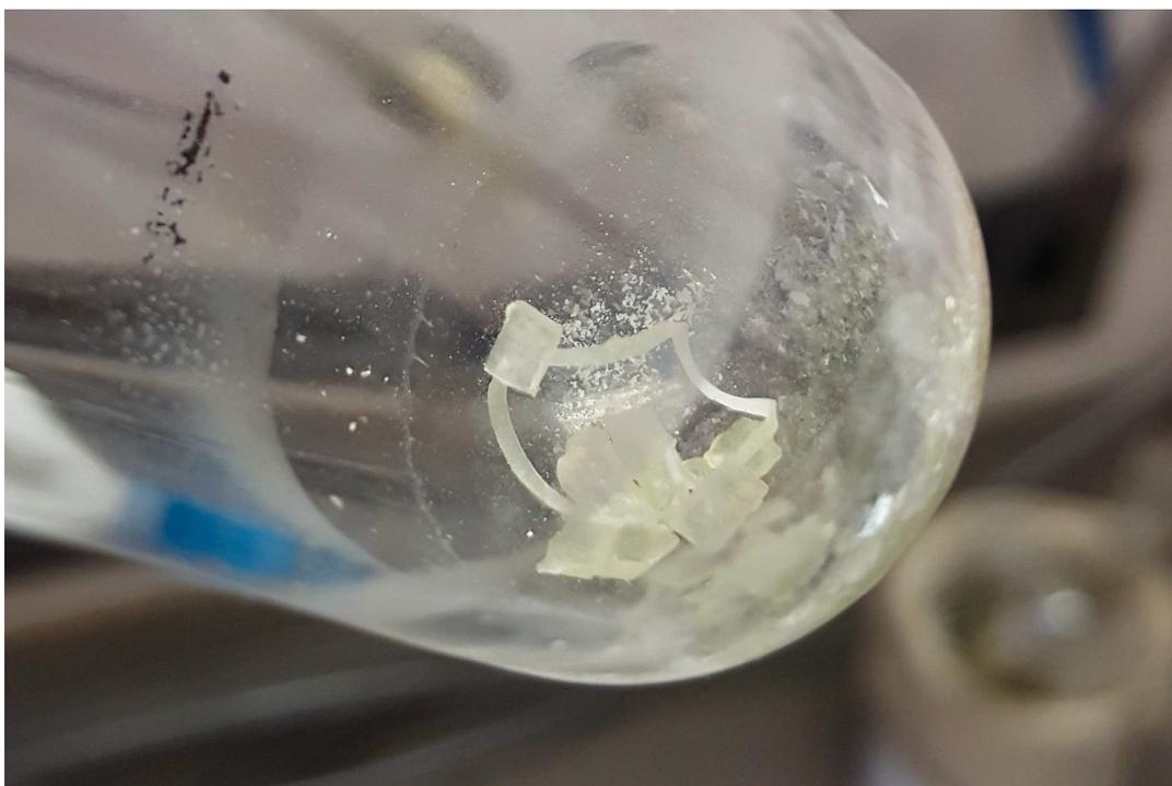
■ **Abb. 61:** Crystals of **3** after removal of the mother liquor and drying in vacuum, with Teflon ring at the bottom of the ampoule for size comparison. The monoclinic crystals reach a size of about 2–3 mm. The growth of crystals of this size required three months.
