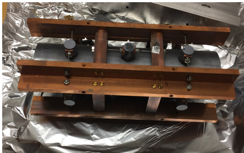
Figure 2.5: Top and middle panels: spacer and the small cylinders before and after completion of the gluing process. Bottom panel: the resonator mounted inside the frame without front plates.
