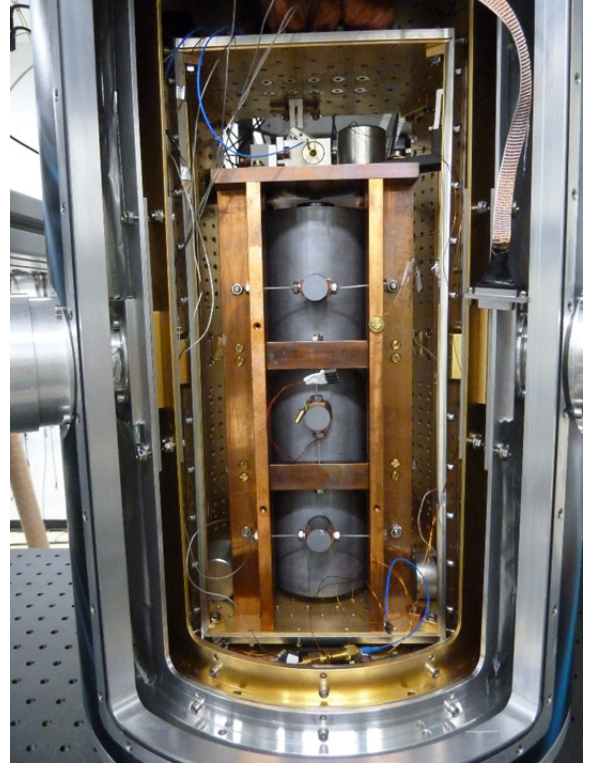
Figure 4.1: Left panel: first cryogenic operation of the vertically-oriented resonator inside a 4 K pulse-tube cryostat with the room-temperature optical setup seen below the cryostat. Right panel: another installation of the vertically-oriented resonator inside a 1.5 K pulse-tube cryostat that did not went to the cryogenic operation due to the insufficient cryostat performance.
