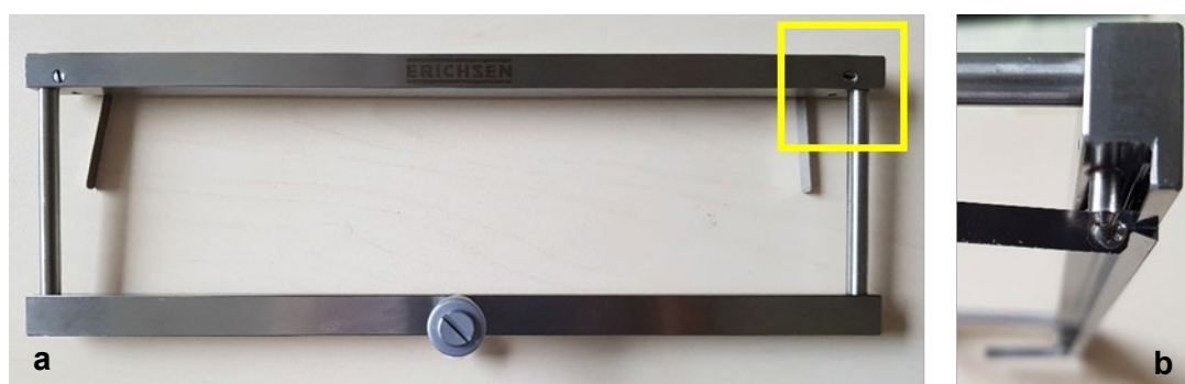
Figure 77: Coating knife (Erichsen) (a) and detailed side view of the wedge-shaped blade geometry (b)
