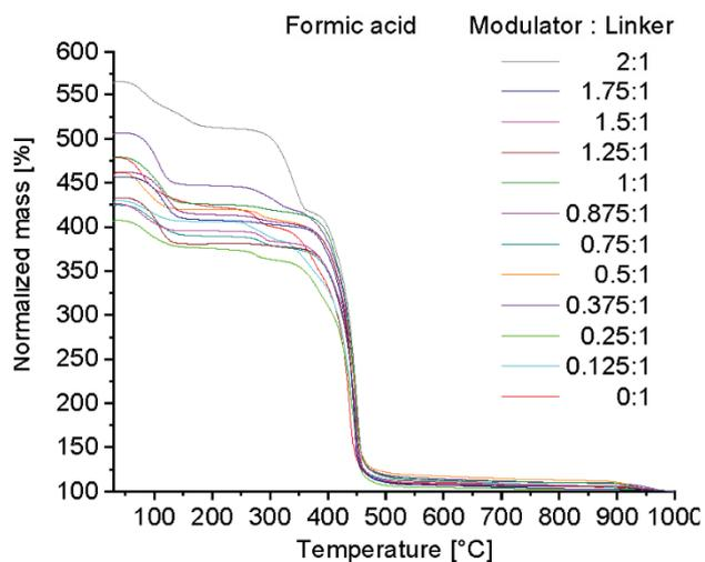
**Figure S17.** TGA measurements of MIL-160 with formic acid as modulator and different modulator : metal/linker ratios. The TGA traces are normalized such that the end mass is 100%.
