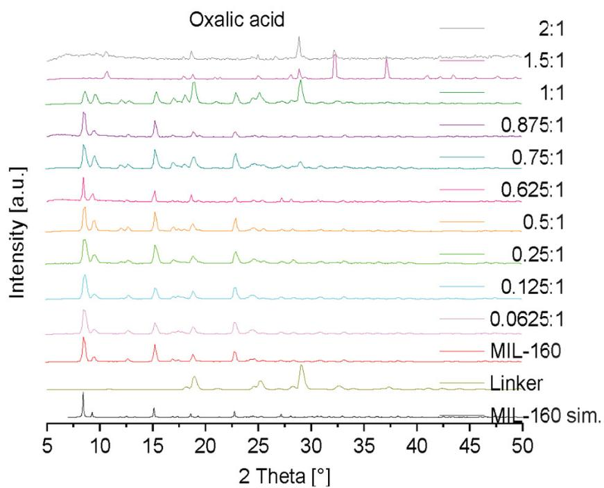
**Figure S8.** PXRDs of oxalic acid modulated MIL-160 for different molar modulator:linker. The simulated diffractogram for MIL-160 is based on the deposited cif file with CCDC no. 1828694, Refcode *PIBZOS*.<sup>6</sup>
