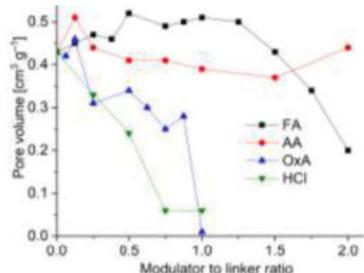
**Figure 3.** Trends of the total pore volume of MIL-160, depending on the modulator to linker ratio of the different modulators. The numbers on the x-axis are always in relation to 1 with respect to the linker amount. The graphs include the values from all tested modulator/linker ratios as given in Table S2-S5, SI.
