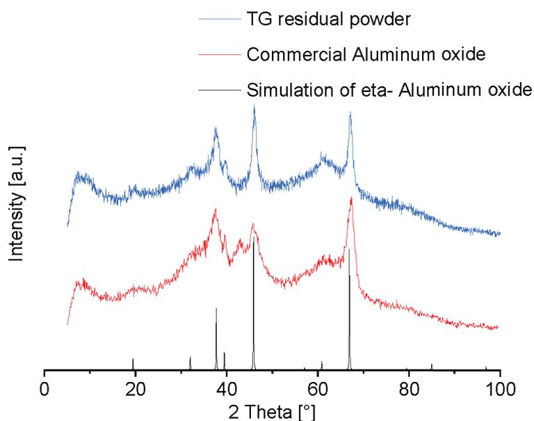
**Figure S14.** Comparison of the residue of MIL-160 after combustion in the TGA crucible, a commercial Al<sub>2</sub>O<sub>3</sub> sample and a simulation of eta-Al<sub>2</sub>O<sub>3</sub>.<sup>7</sup>
