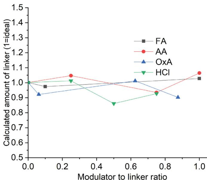
**Figure S24.** Trends of the linker amounts of MIL-160, depending on the modulator to linker ratio of the different modulators. The numbers on the x-axis are always in relation to 1 with respect to the linker amount.
