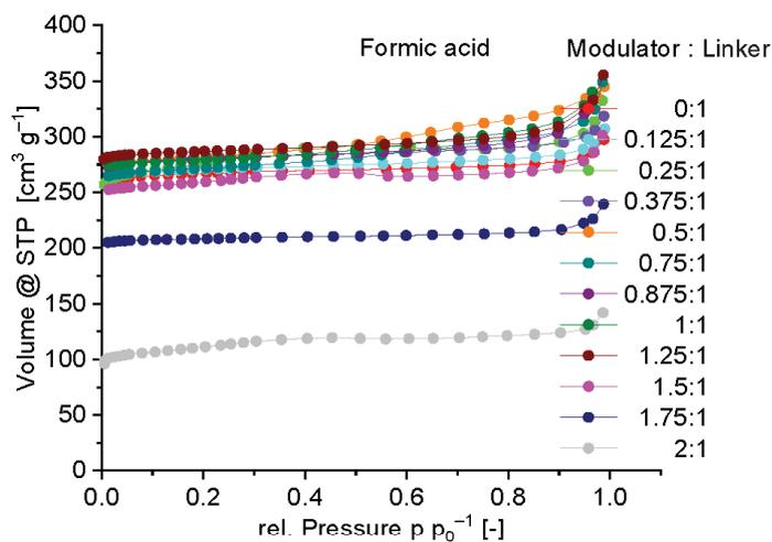
**Figure S2.** Nitrogen adsorption isotherms of formic acid modulated MIL-160 at 77 K. For clarity, the desorption isotherms are not shown.
