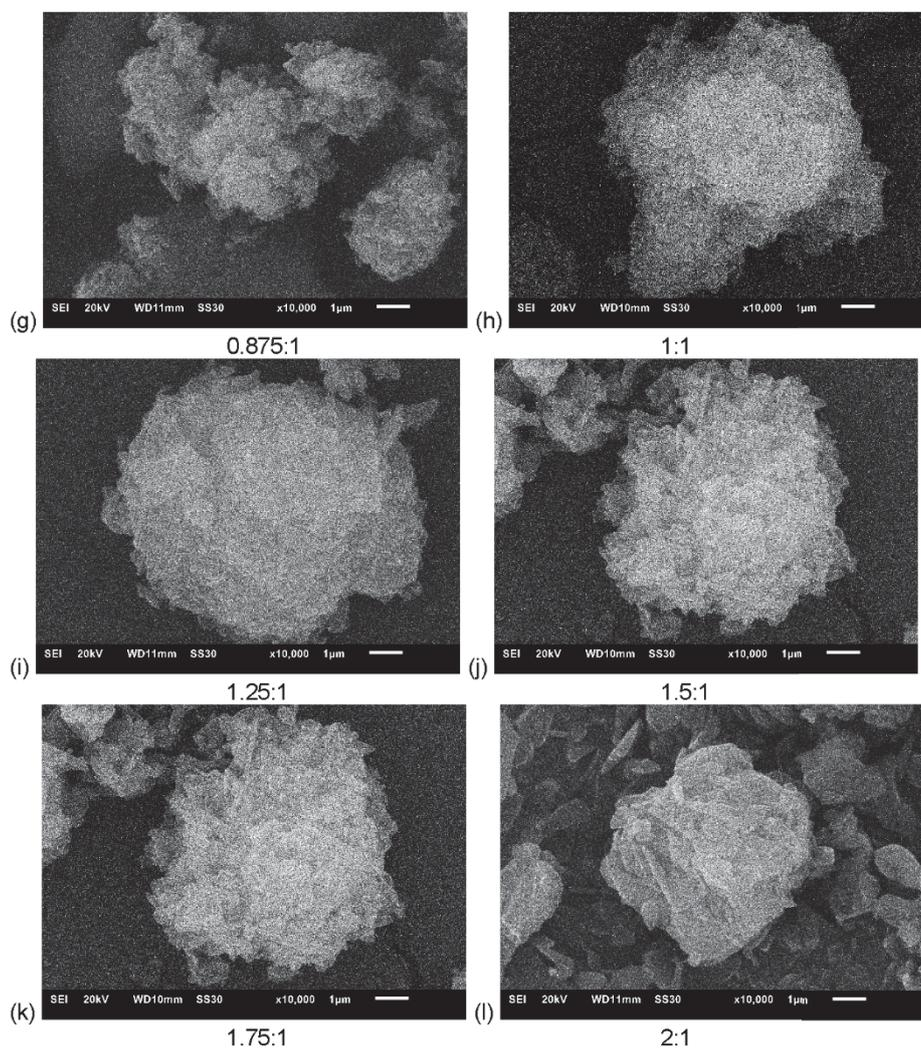
**Figure 21.** Formic acid modulated MIL-160 series with modulator to linker ratios of (a) unmodulated MIL-160, (b) 0.125:1, (c) 0.25:1, (d) 0.375:1, (e) 0.5:1, (f) 0.775:1, (g) 0.875:1, (h) 1:1, (i) 1.25:1, (j) 1.5:1, (k) 1.75:1 and (l) 2:1. The ratios are also given under each SEM picture.
