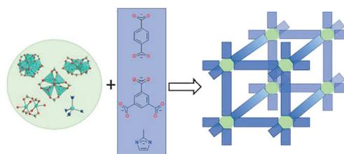
Figure 1. Construction principle of MOFs from metal clusters or metal atoms (examples shown with their attached donor atoms from ligands with carboxylate,  $-\text{CO}_2$  or azolate,  $-\text{N}$  groups) and organic ligands (linkers) into a three-dimensional porous framework.
