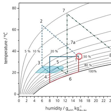
Figure 14. Process paths of a solid desiccant cooling (SDC) system (---) and of a desiccant and evaporative cooling (DEC) system (—; ingoing air, —: outgoing air) are depicted in comparison to a conventional A/C system (\*) in a Mollier diagram.
