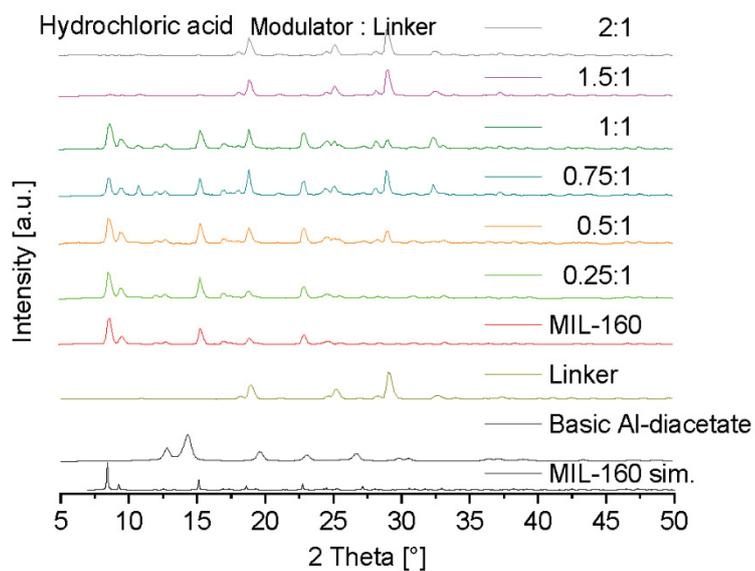
**Figure S9.** PXRDs of hydrochloric acid modulated MIL-160 for different molar modulator:linker. The simulated diffractogram for MIL-160 is based on the deposited cif file with CCDC no. 1828694, Refcode *PIBZOS*.<sup>[6]</sup>
