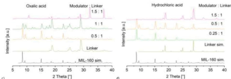
**Figure 1.** Selected powder X-ray diffraction patterns of MIL-160 synthesized with different modulators and molar modulators:linker ratios as indicated. The simulated diffractogram for MIL-160 is based on the deposited of file with CCDC no. 1828894, Refcode PIBZOS.<sup>[28]</sup> The simulated diffractogram for the linker is based on the deposited of file with CCDC no. 11611468, Refcode FURDCA.<sup>[29]</sup> For diffraction patterns for all used modulator:linker ratios see Fig. S6-S9, SI.
