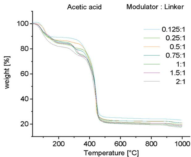
**Figure S18.** TGA measurements of MIL-160 with acetic acid as modulator and different modulator:metal/linker ratios.
