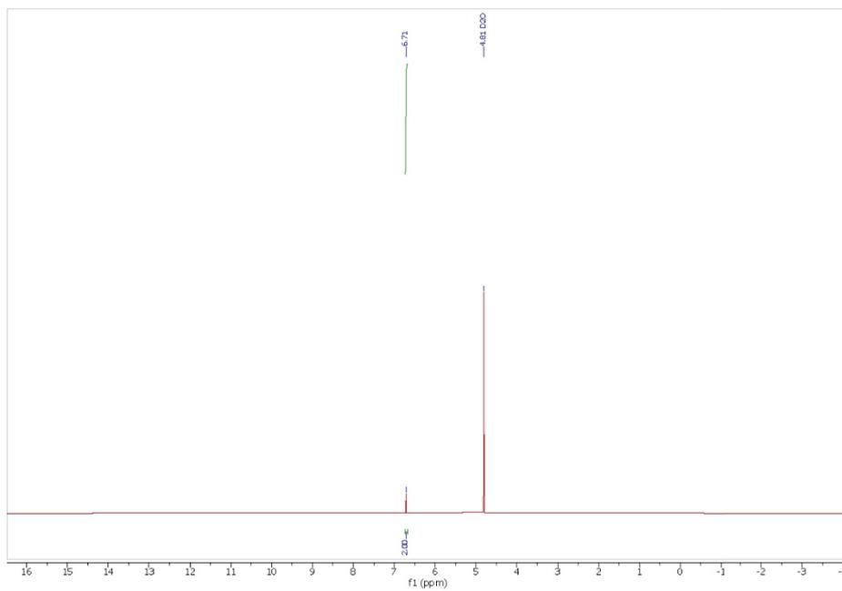
**Figure S11.**  $^1\text{H}$  NMR spectrum of "digested" MIL-160, modulated with acetic acid at a molar modulator:metal/linker ratio of 2:1, after decomposition with 5% NaOD/D<sub>2</sub>O, in D<sub>2</sub>O. The furandicarboxylate linker signal appears at 6.59 ppm (normalized to two protons), the solvent signal at 4.79 ppm.
