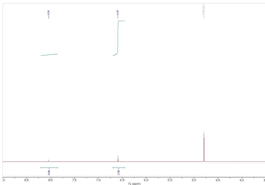
**Figure S12.**  $^1\text{H}$  NMR spectrum of "digested" MIL-160, modulated with acetic acid at a molar modulator:metal/linker ratio of 2:1, after decomposition with 5% NaOD/D<sub>2</sub>O. The furandicarboxylate linker signal appears at 6.59 ppm (normalized to two protons), the formate signal at 8.04 ppm, the solvent signal at 4.79 ppm.
