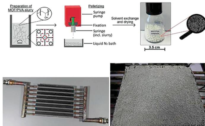
Figure 12. Top: freeze granulation process of MOF/polyvinyl alcohol (PVA) composites. Bottom: pipe-lamella heat exchanger unfilled (left) and filled (right) with pellets.<sup>[31]</sup> Reproduced from ref.<sup>[30]</sup> © (2019), with permission from the American Chemical Society.
