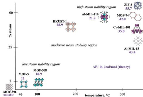
Figure 8. Hydrothermal stability of different MOFs against water vapor at different temperatures as a steam–temperature diagram. The corresponding activation energies for the MOFs, which are required for the exchange of a linker, are plotted as numerical values. Reproduced from ref.<sup>[92]</sup> © (2009), with permission from the American Chemical Society.
