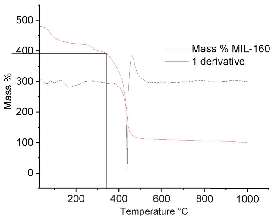
Figure S20. TGA measurement of MIL-160. The black lines show the chosen point for defect determination.
