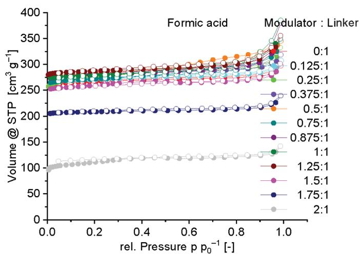
**Figure S2.1.** Nitrogen sorption isotherms of formic acid modulated MIL-160 at 77 K. Desorption is shown as empty dots of the same color as the sorption.
