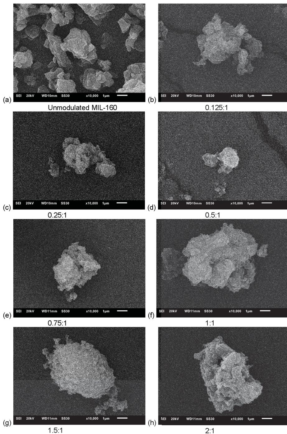
**Figure S22.** Acetic acid modulated MIL-160 series with modulator to linker ratios of (a) unmodulated MIL-160, (b) 0.125:1, (c) 0.25:1, (d) 0.5:1, (e) 0.75:1, (f) 1:1 and (g) 1.5:1 and (h) 2:1. The ratios are also given under each SEM picture.
