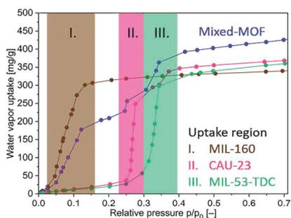
Figure 11. Comparison of uptake regions and water uptake from MIL-160, CAU-23, MIL-53-TDC, and the Mixed-MOF (purple-blue), containing a near 1:1 mixture of the TDC and FDC linker.<sup>[100]</sup> Reproduced from ref.<sup>[80]</sup> © (2019), with permission from the Royal Society of Chemistry.
