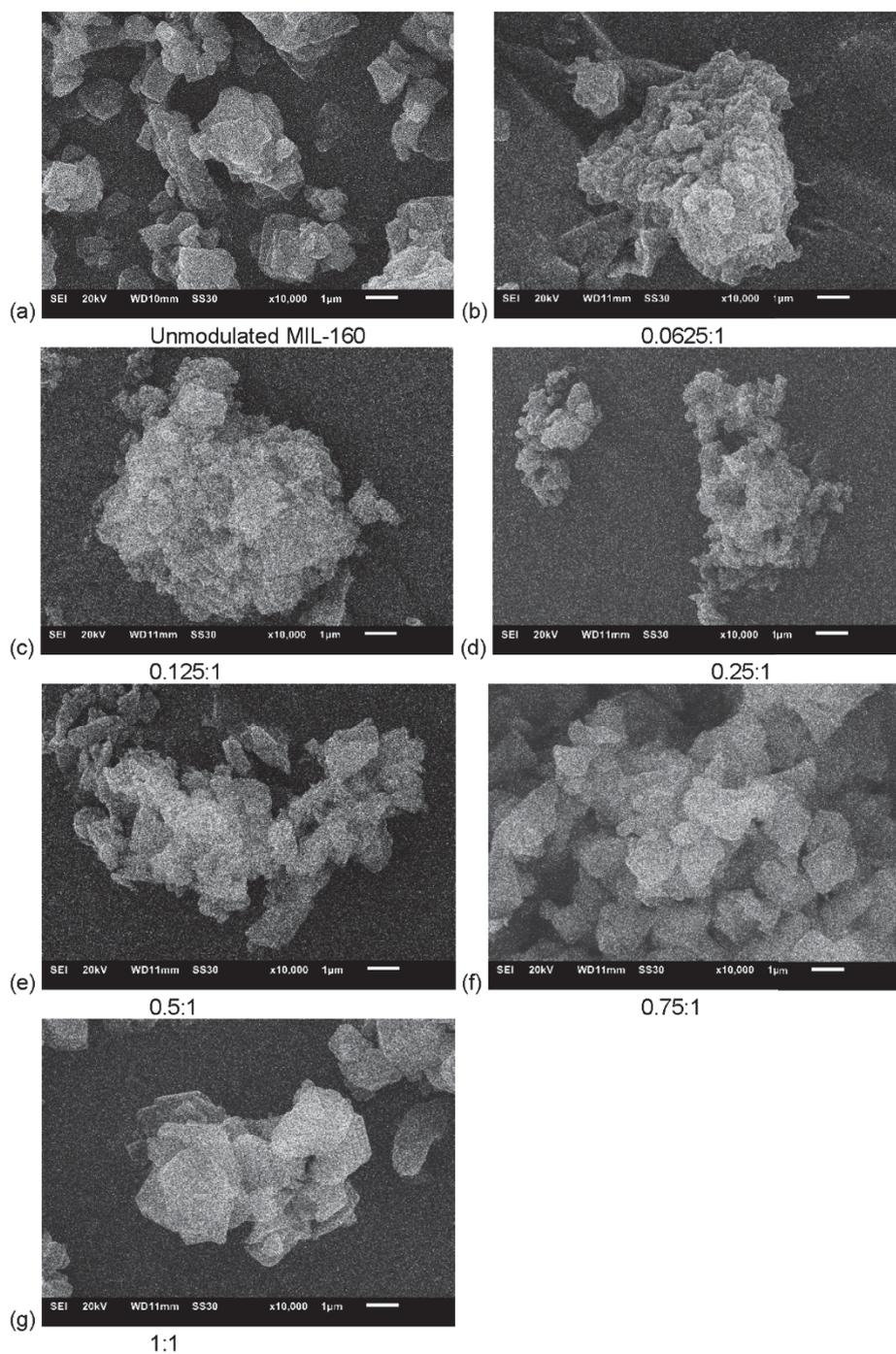
**Figure S23.** Oxalic acid modulated MIL-160 series with modulator to linker ratios of (a) unmodulated MIL-160, (b) 0.0625:1, (c) 0.125:1, (d) 0.25:1, (e) 0.5:1, (f) 0.75:1 and (g) 1:1. The ratios are also given under each SEM picture.
