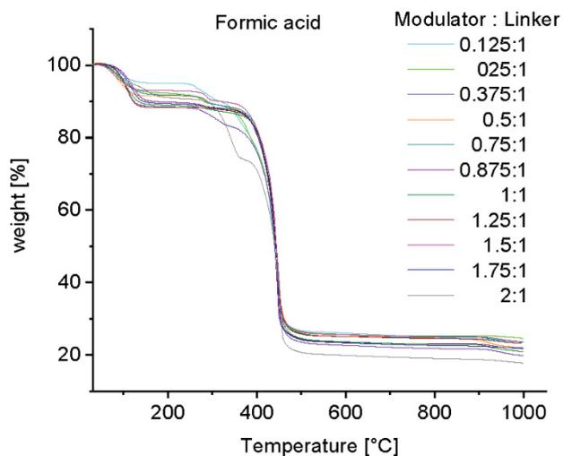
**Figure S16.** TGA measurements of MIL-160 with formic acid as modulator and different modulator: metal/linker ratios.
