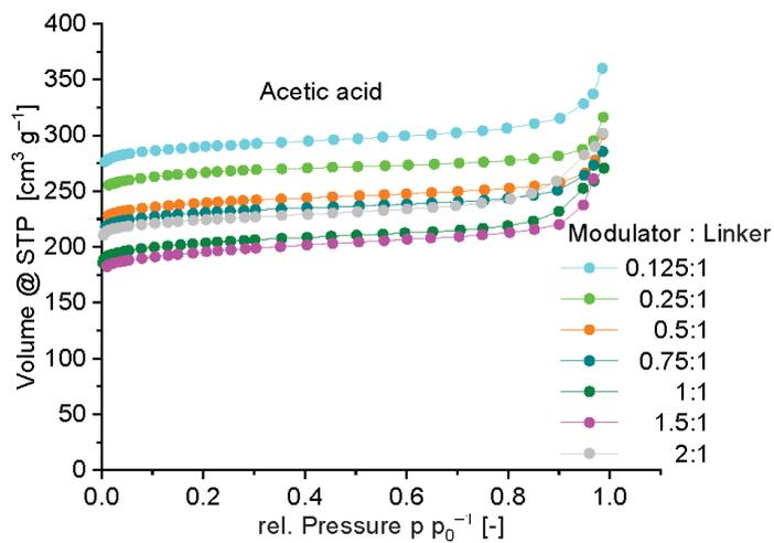
**Figure S3.** Nitrogen adsorption isotherms of acetic acid modulated MIL-160 at 77 K. For clarity, the desorption isotherms are not shown.
