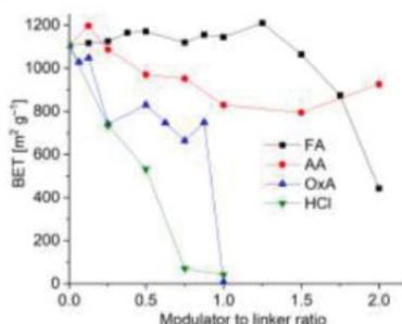
**Figure 2.** Trends of the BET surface of MIL-160, depending on the modulator to linker ratio of the different modulators. The numbers on the x-axis are always in relation to 1 with respect to the linker amount. The graphs include the values from all tested modulator/linker ratios as given in Table S2-S5, SI.
