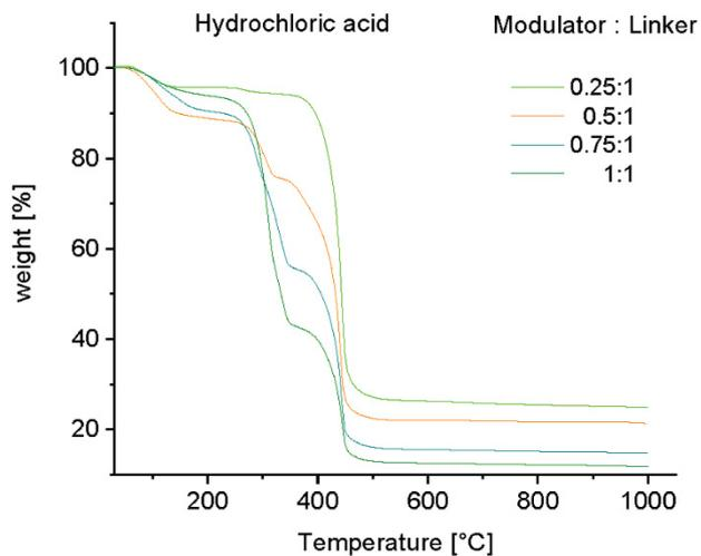
**Figure S22.** TGA measurements of MIL-160 with hydrochloric acid as modulator and different modulator:metal/linker ratios.
