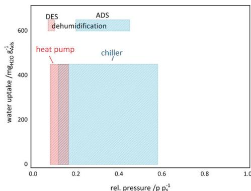
Figure 15. Working windows of possible application based on water adsorption.
