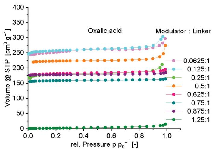
**Figure S4.** Nitrogen adsorption isotherms of oxalic acid modulated MIL-160 at 77 K. For clarity, the desorption isotherms are not shown.
