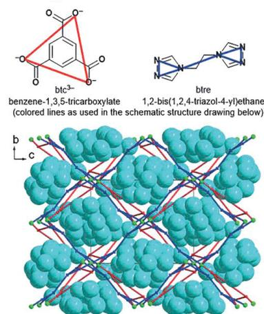
Figure 5. Schematic drawing of the 3D framework 3D-[(Ni<sub>3</sub>(μ<sub>3</sub>-btc)<sub>2</sub>(μ<sub>4</sub>-btre)<sub>2</sub>(μ-H<sub>2</sub>O)<sub>2</sub>]<sub>n</sub>·ca. 22H<sub>2</sub>O} (btc ligand in red, btre ligand in dark blue, nickel atoms in green) with the oxygen atoms (light blue) of the water of crystallization in space-filling mode.<sup>[69,70]</sup> Reproduced from ref.<sup>[70]</sup> © (2009), with permission of the American Chemical Society.
