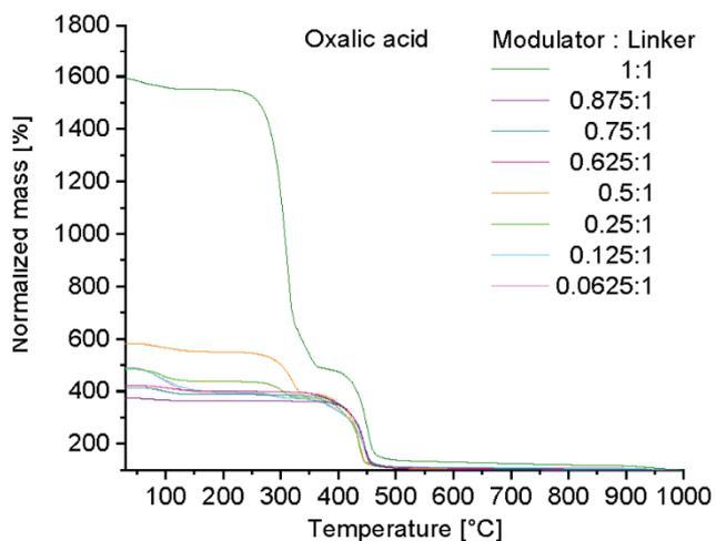
**Figure S21.** TGA measurements of MIL-160 with oxalic acid as modulator and different modulator:metal/linker ratios. The TGA traces are normalized such that the end mass is 100%.
