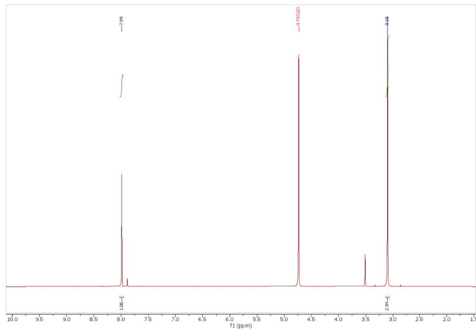
**Figure S13.** <sup>1</sup>H NMR spectrum of formic acid and methanol at a molar ratio of 1:1 after decomposition with 5% NaOD, in D<sub>2</sub>O, the formate signal appears at 8.04 ppm, the methanolate signal at 3.10 ppm, the solvent signal at 4.79 ppm.
