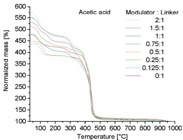
**Figure S19.** TGA measurements of MIL-160 with acetic acid as modulator and different modulator:metal/linker ratios. The TGA traces are normalized such that the end mass is 100%.
