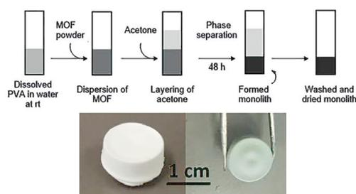
Figure 13. Top: schematic fabrication procedure of MOF/PVA monoliths via phase separation. Bottom: photographic images of Al-fum50/PVA2 (left) and MIL-101(Cr)40/PVA1 monolith (right).<sup>[120]</sup> Reproduced from ref.<sup>[100]</sup> © (2019), with permission from Elsevier.
