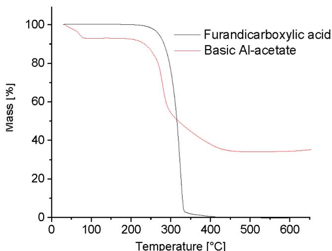
**Figure S15.** TG measurement of the MIL-160 educts.
