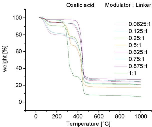
**Figure S20.** TGA measurements of MIL-160 with oxalic acid as modulator and different modulator:metal/linker ratios.
