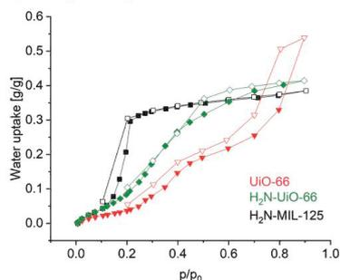
Figure 9. Water adsorption/desorption isotherms of UiO-66 (red), H<sub>2</sub>N-UiO-66 (green) and H<sub>2</sub>N-MIL-125 (black), acquired at T = 25 °C.<sup>[81]</sup> Adsorption: filled symbols; desorption: empty symbols.
