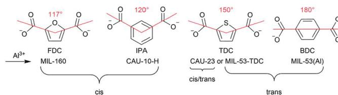
Scheme 1. Schematic illustration of linker molecules relevant in this work, their opening angles, and the resulting MOFs with their *cis*- and/or *trans*-( $\mu$ -OH)<sub>2</sub> connectivity of the  $\{\text{Al}(\text{OH})_2(\text{O}-\text{C}-\text{O})_4\}$  octahedra.
