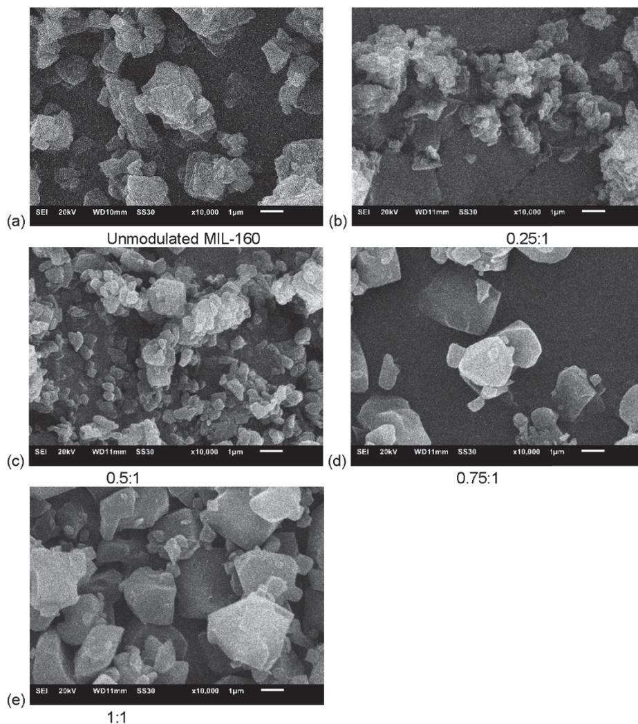
**Figure S24.** Hydrochloric acid modulated MIL-160 series with modulator to linker ratios of (a) unmodulated MIL-160, (b) 0.25:1, (c) 0.5:1 (d) 0.75:1 and (e) 1:1. The ratios are also given under each SEM picture.
