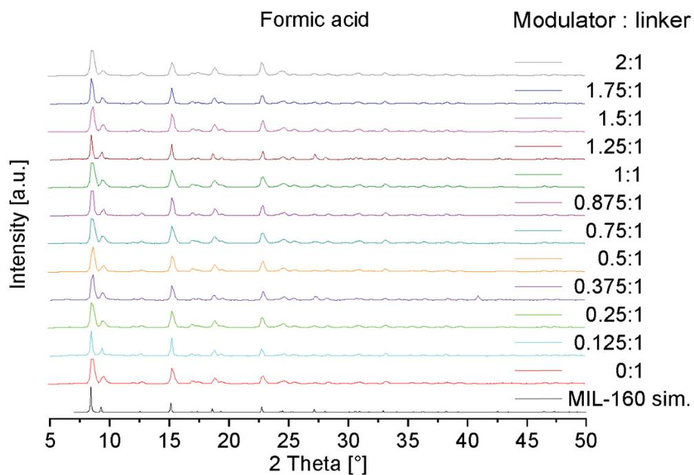
**Figure S6.** PXRDs of formic acid modulated MIL-160 for different molar modulator:linker. The simulated diffractogram for MIL-160 is based on the deposited cif file with CCDC no. 1828694, Refcode *PIBZOS*.<sup>6</sup>
