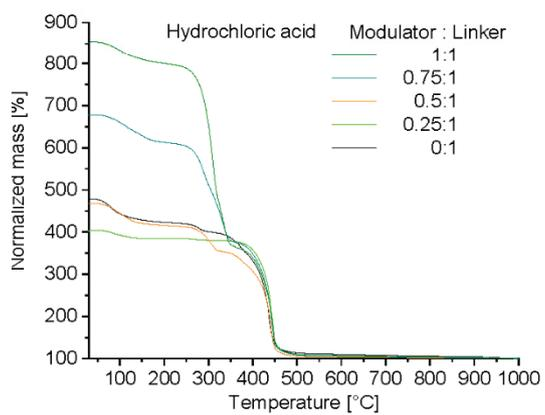
**Figure S23.** TGA measurements of MIL-160 with hydrochloric acid as modulator and different modulator:metal/linker ratios. The TGA traces are normalized such that the end mass is 100%.
