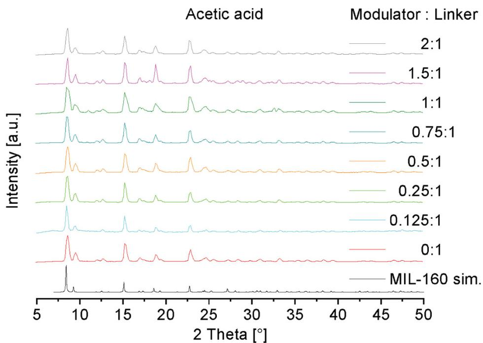
**Figure S7.** PXRDs of acetic acid modulated MIL-160 for different molar modulator:linker. The simulated diffractogram for MIL-160 is based on the deposited cif file with CCDC no. 1828694, Refcode *PIBZOS*.<sup>6</sup>
