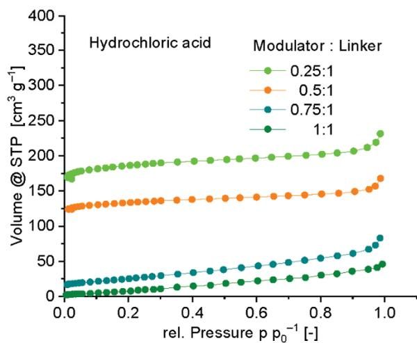
**Figure S5.** Nitrogen adsorption isotherms of hydrochloric acid modulated MIL-160 at 77 K. For clarity, the desorption isotherms are not shown.
