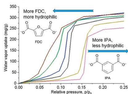
Figure 10. Fine-tuning of water adsorption curves with solid solution mixed-linker aluminum MOFs with varying furandicarboxylate and isophthalate linker proportions between (from left to right) neat MIL-160 (FDC-only, brown), IPA:FDC 22:78 (green), 53:47 (blue), 74:26 (grey), 85:15 (olive), neat CAU-10-H (IPA only, pink).<sup>[101]</sup> Reproduced from ref.<sup>[81]</sup> © (2019), with permission the American Chemical Society.
