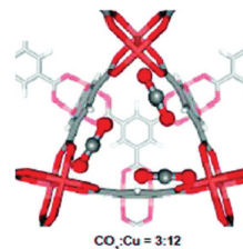
Fig. 28 Structure of the CO 2 adsorption complexes on the Cu 2+ site for CO 2 /Cu coverage of 3 : 12. Reproduced from ref. 232 with permission from the American Chemical Society, copyright 2011.
