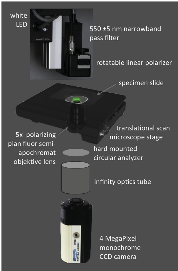
Fig. 3 – Hardware setup of the polarization microscope.
